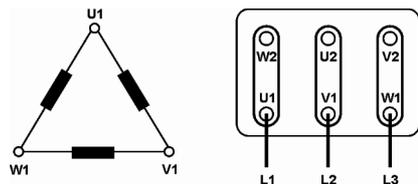
Delta connection is obtained by connecting the end of a phase to the beginning of the next phase.
