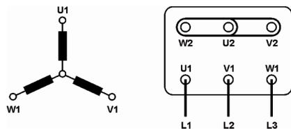
Star connection is obtained by connecting terminals W2, U2, V2 to each other and terminals U1, V1, W1 to the mains.
